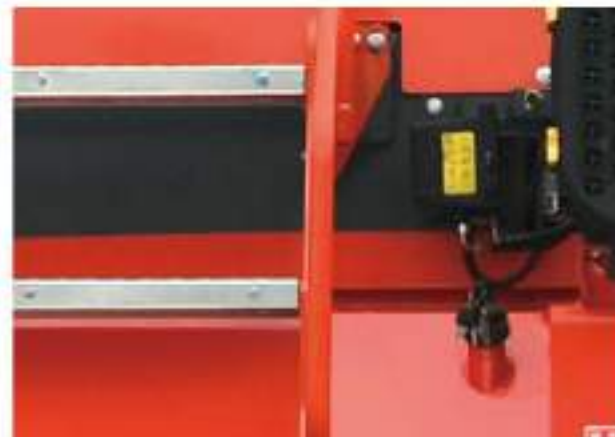
• Electric tilting button with high dust-proof and water-proof degree: protecting degree:IP67
