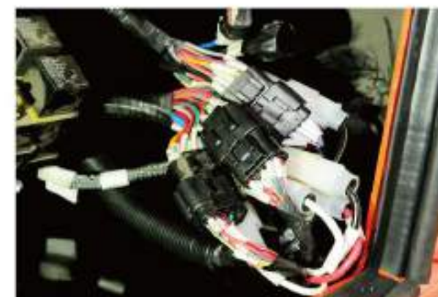
• Dust-proof waterproof connectors: protective class IP65
